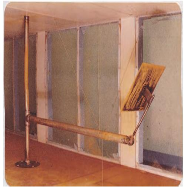
Fig. 6a. Surface flow visualization setup
